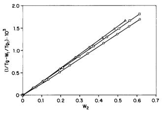
**Figure 4** Comparison of the theoretical  $T_g$  values calculated from the Fox equation to the experimental  $T_g$  values of PVC copolymers obtained by melt modification:  $\bigcirc$ , VC-VTB;  $\triangle$ , VC-VTC;  $\square$ , VC-VTN
